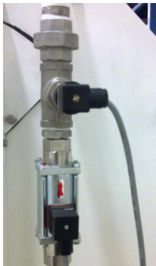
Photo 8: Suco pressure transmitter (above) and water valve (below)
